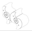
DS150 is a single stage dry claw, direct driven and air-cooled vacuum pump. The pump is designed in modular construction concept having two compartments; pumping area and gear box, separated by a piston ring and rotary shaft seals. Pump inlet port is protected by a metal wire mesh strainer to safe guard pump from entry of solid particle.
